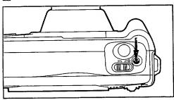
Press the macro button ( ) to engage the Macro mode, and the lens moves forward. To cancel the Macro mode, just move the zooming lever to the left ( ) or right ( ). The ordinary shooting mode is then restored.
