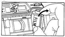
Open the back cover, and remove the cartridge from the chamber by pulling on its top with your fingertip as shown.
