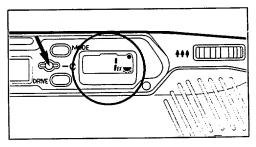
When the LCD panel is as shown above, the camera is in the Auto and Single-Frame Shooting modes. These modes are used for ordinary picture-taking situations. If the LCD panel displays indications other than those above, press the mode drive clear (  $\mathbf{C}$  ) button to reset the LCD panel to appear as above.
