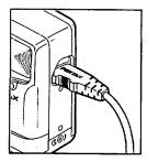
When shooting using the Bulb modes, use a tripod. The optional Cable Switch F can be used by inserting it into the release socket.
