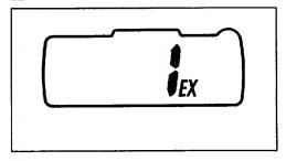
When "1" appears in the exposure counter on the LCD panel, the film automatically stops winding. The indication as shown above appears.
