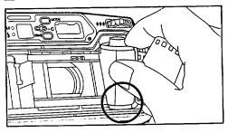
Place the film cartridge in the film chamber, fitting its flat side on the top of the rewind shaft.
