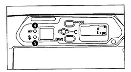
When you press the shutter release button half-way, the lamps (a) and/or (5) as shown above glow or flicker.
