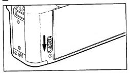
Slide the back cover release lever in the direction of the arrow as illustrated to open the back cover. 2
