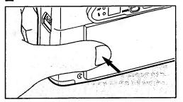
Close the back cover. The film automatically advances to the first frame. (Even if no film is loaded, the motor operates for a second or two after the back cover is closed.) 5
