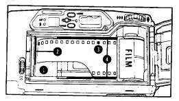
Pull the film leader out far enough from the cartridge to reach the take-up spool ●. Align the tip with the film leader end mark ●.
