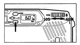
To select the shooting interval, while pressing the drive button, press the zooming lever to the left or right until the required interval time appears on the LCD panel. The preset interval time is 60 seconds. (When the zooming lever is kept depressed, the interval time will be fast forwarded.)
