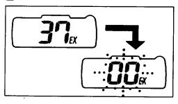
After you have exposed the last frame of the roll, film rewinds automatically. Then, the motor stops, and ( OO) flickers as shown to indicate end of rewind. 2
